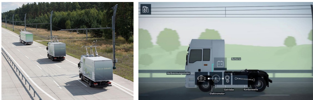
Figure 1. Siemens Mobility eHighway & Hybrid drivetrain ( https://new.siemens.com/global/en/products/mobility/road-solutions/electromobility/ehighway.html )
